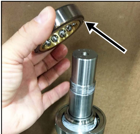
Figure 176 - Place bearing onto race
