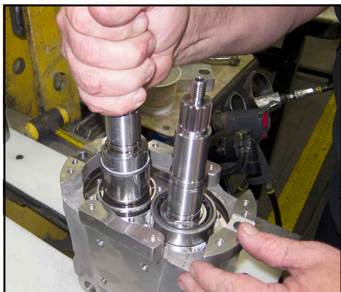
Figure 199 - Place drive shaft in bore
