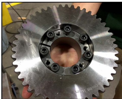
Figure 223 - Place locking assembly into gear
