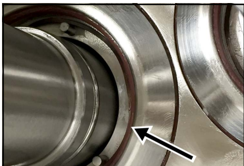
Figure 49 - Remove carrier-to-seal O-ring
