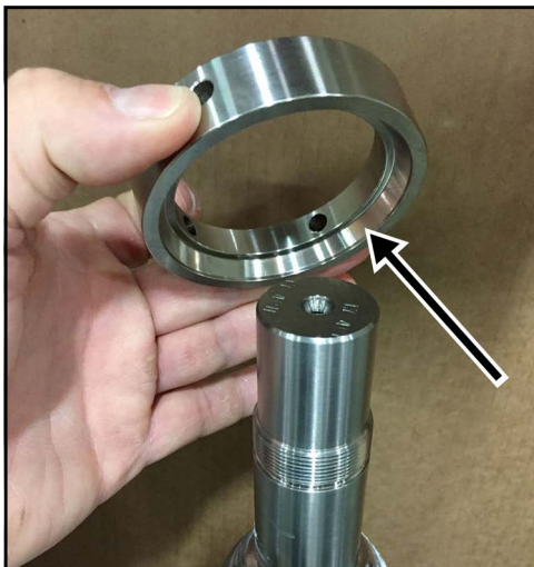
Figure 168 - Place bearing spacer on shaft
