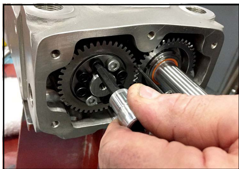
Figure 150 - Loosen bolts in locking assembly
