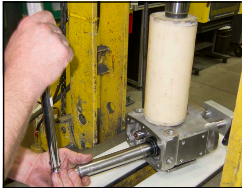
Figure 218 - Torque locking nut
