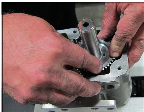
Figure 214 - Install drive gear
