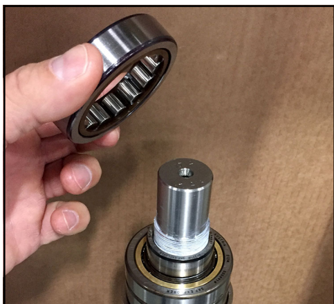
Figure 188 - Place bearing onto race
