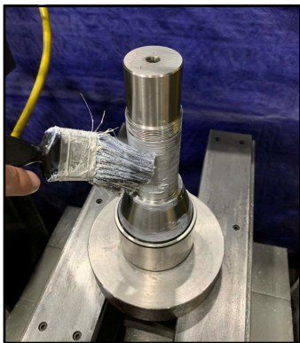
Figure 279 -Apply anti-seize to shaft
