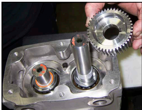
Figure 213 - Install drive gear
