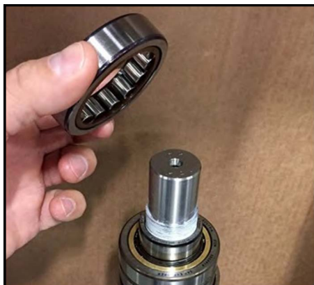
Figure 288 -Place bearing onto race
