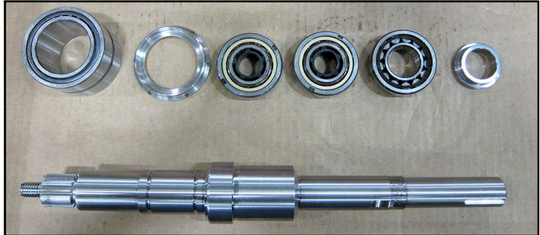
Figure 161 - Drive Shaft: Assembly items needed
