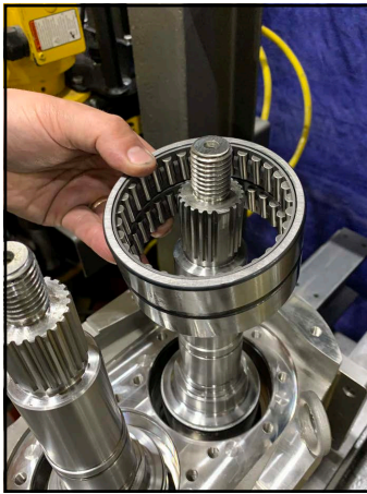
Figure 313 -Place outer race on the shafts
