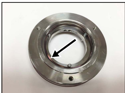
Figure 74 - Seal wave spring installed
