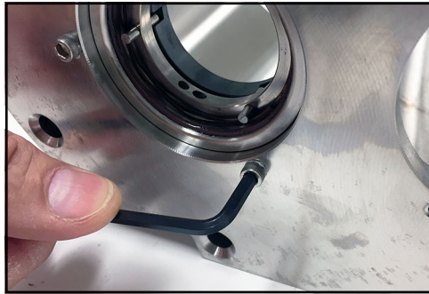
Figure 56 - Remove cap screws
