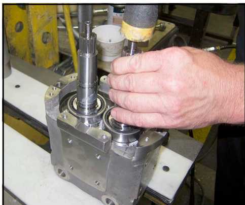
Figure 201 - Tap shafts to center in bores
