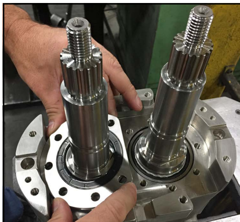
Figure 210 - Install bearing retainer
