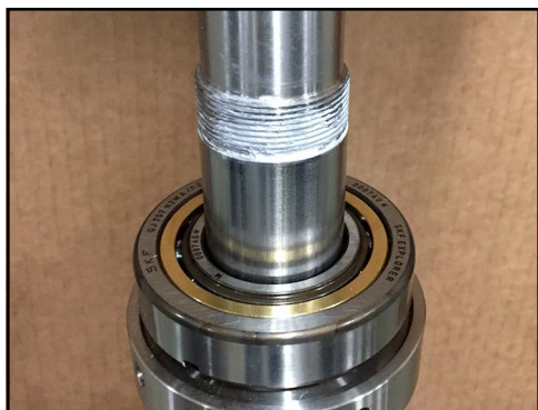
Figure 178 - Race installed on shaft
