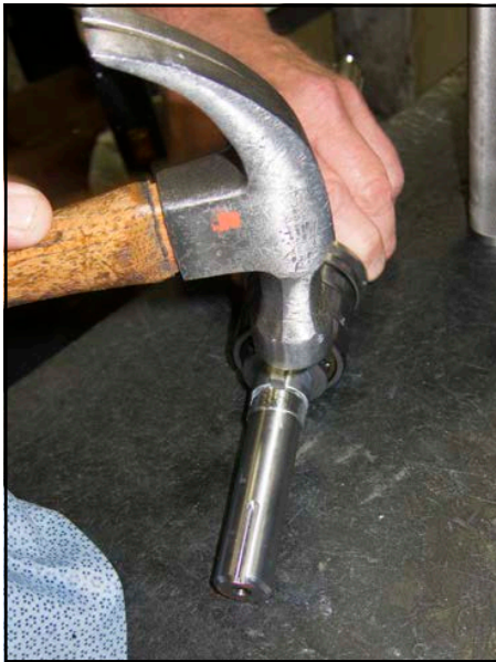
Figure 301 -Tap key into key way
