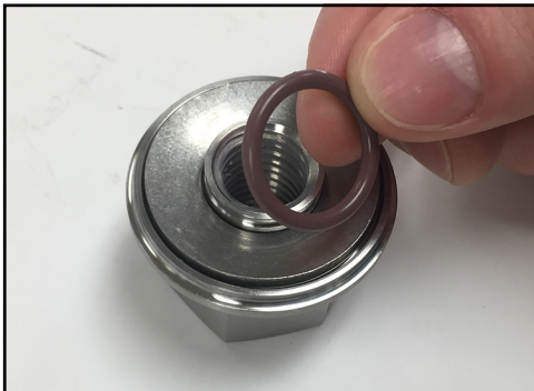
Figure 39 - Remove washer retainer O-ring
