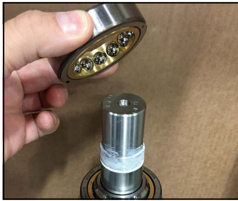
Figure 181 - Place bearing onto race
