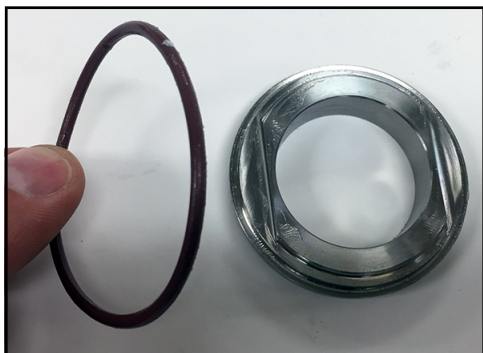
Figure 46 - Remove cap-to-seat O-ring
