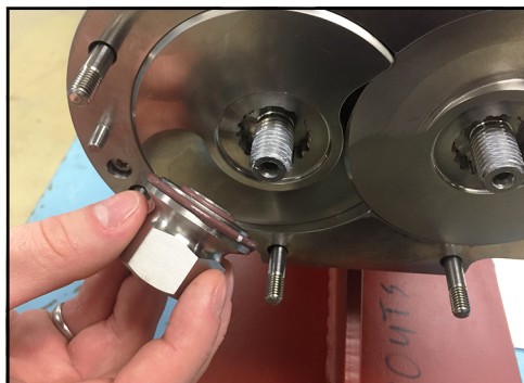
Figure 122 - Install screw nuts
