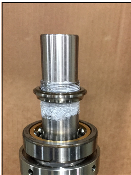
Figure 292 -Place race on shaft
