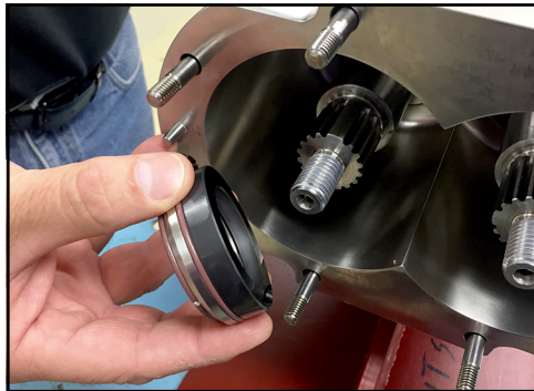
Figure 43 - Remove seal cap assembly
