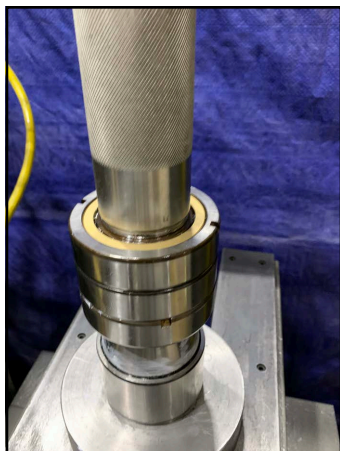
Figure 293 -Press race into bearing
