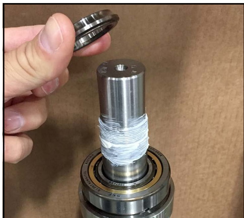
Figure 179 - Place race on shaft
