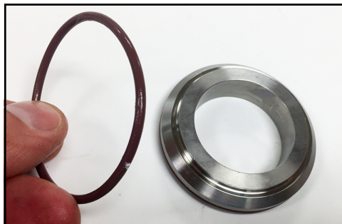
Figure 102 - Install cap-to-screw O-ring
