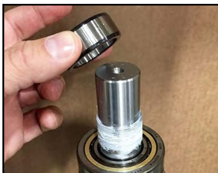
Figure 286 -Place race onto shaft
