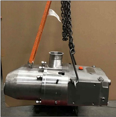
Figure 3 - Lifting location - 130, 220-UTS
