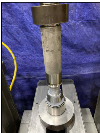
Figure 281 -Press race onto shaft
