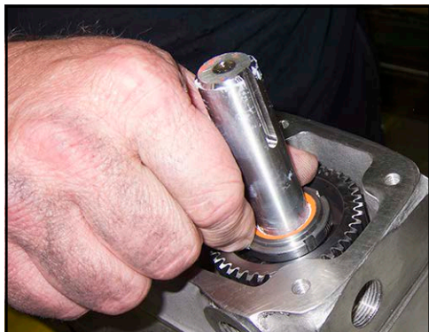
Figure 216 - Install locking nut
