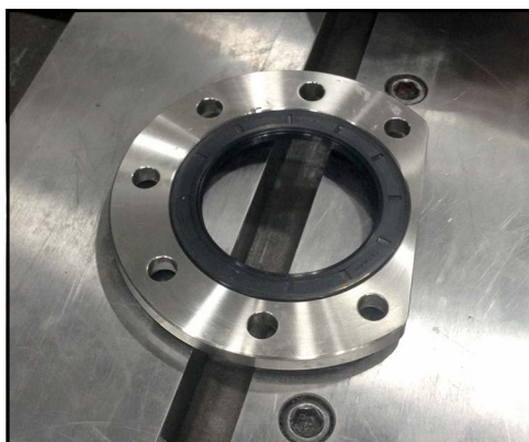
Figure 205 - Bearing retainer seal installed
