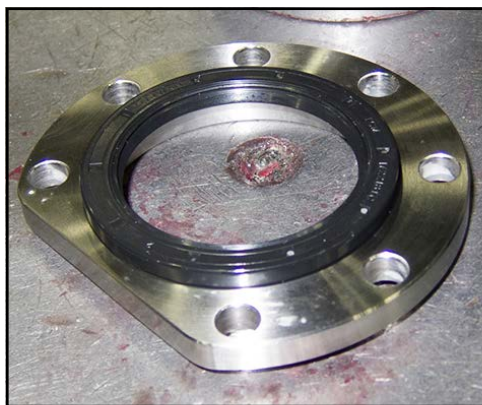
Figure 203 - Center bearing retainer seal
