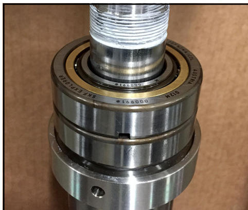
Figure 184 - Second bearing installed
