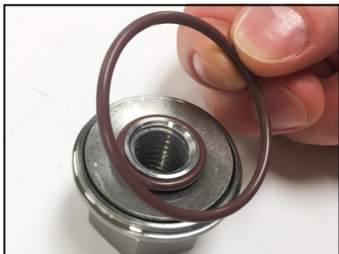
Figure 119 - Install screw nut O-ring
