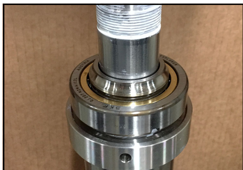
Figure 180 - Press race into bearing
