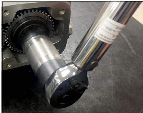
Figure 260 - Loosen locking nut
