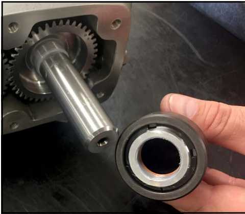
Figure 261 - Remove locking nut and gear
