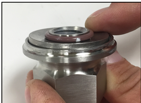
Figure 118 - Belleville washer installed
