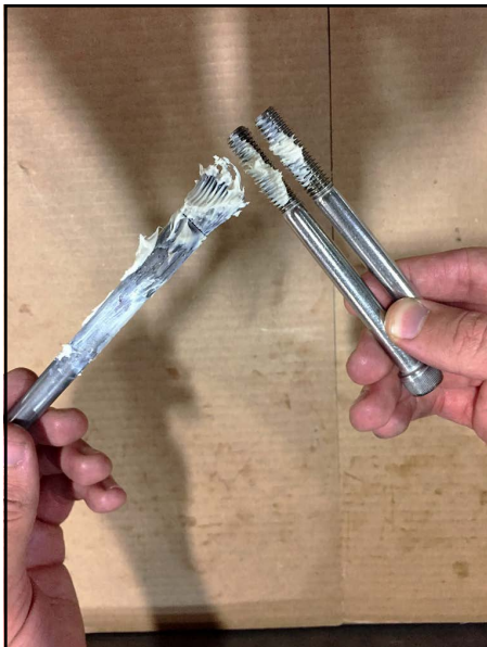
Figure 142 - Apply anti-seize to threads
