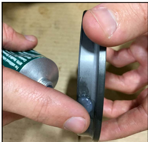
Figure 84 - Lubricate the outer diameter of the seal
