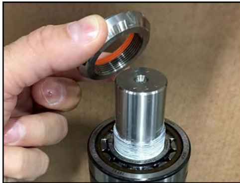
Figure 295 - -Place locking nut onto shaft
