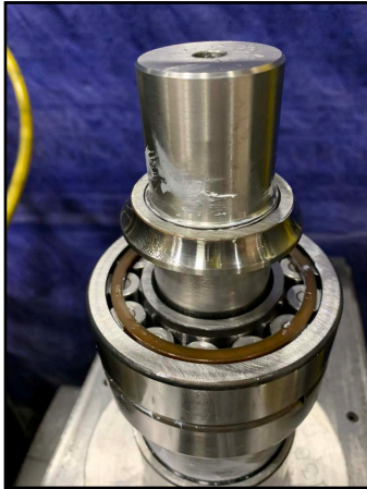
Figure 290 -Press race into bearing
