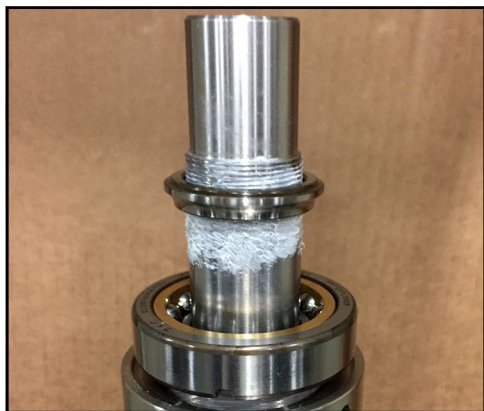
Figure 177 - Place race on shaft
