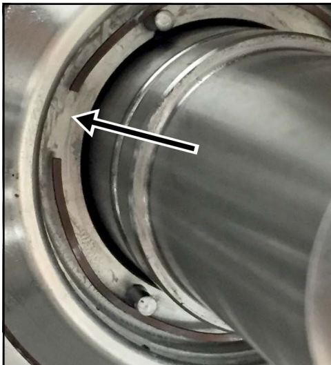
Figure 71 - Seal wave spring position
