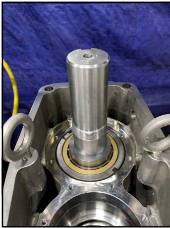
Figure 307 -Place drive shaft in bore
