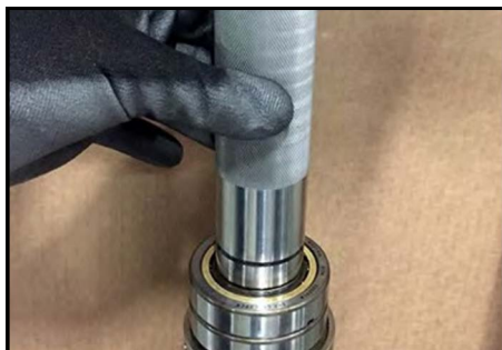
Figure 287 -Press race onto shaft
