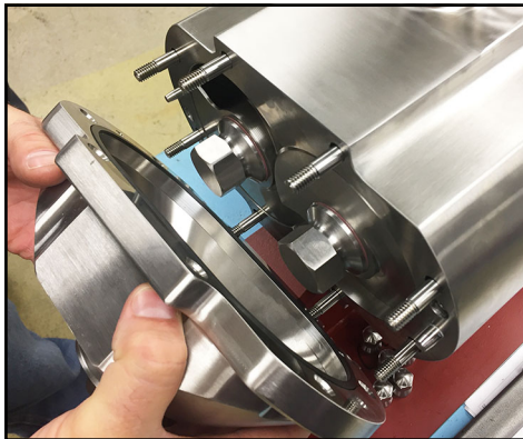
Figure 131 - Install pump cover
