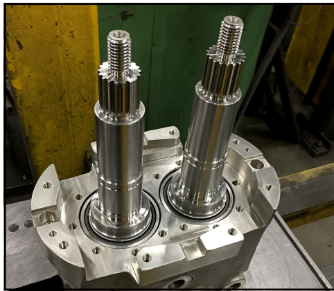
Figure 202 - Shafts seated in gearcase
