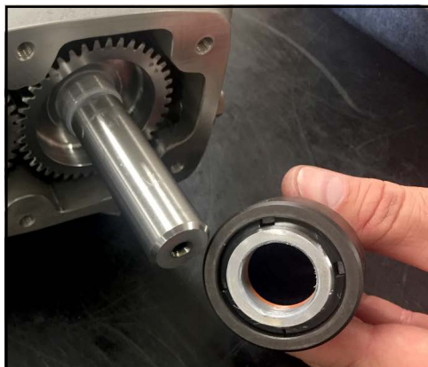
Figure 155 - Remove locking nut and gear
