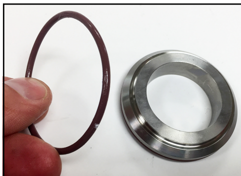
Figure 45 - Remove cap-to-screw O-ring
