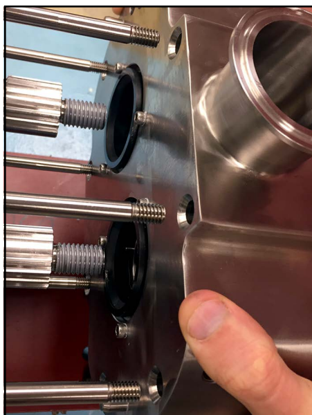
Figure 140 - Install pump body onto shafts
