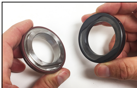
Figure 44 - Remove seal seat from seal cap
