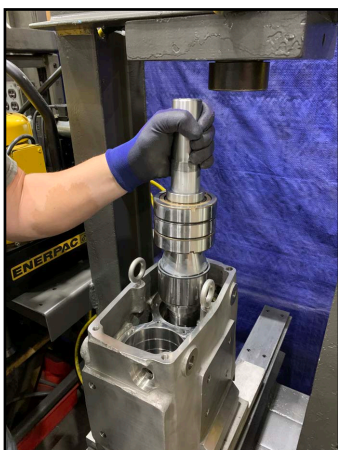
Figure 305 -Place drive shaft in bore
