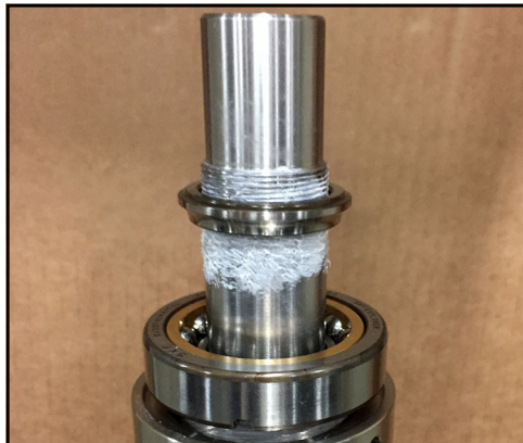
Figure 182 - Place race on shaft
