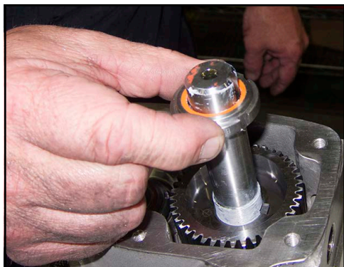
Figure 215 - Install locking nut
