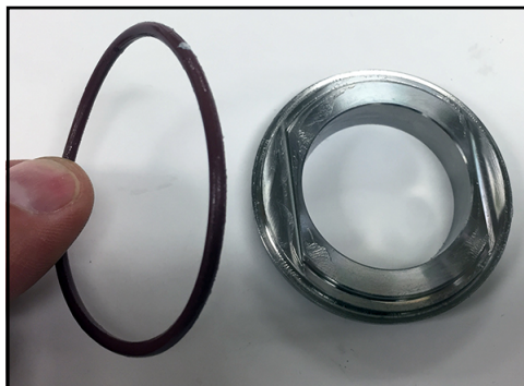
Figure 100 - Install cap-to-seat O-ring
