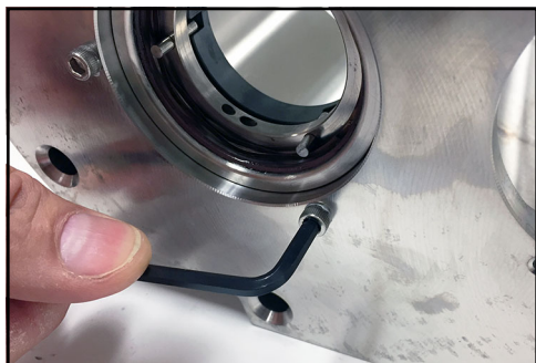
Figure 83 - Install with cap screws
