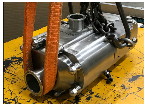
Figure 2 - Lifting location detail - 015, 030-UTS
