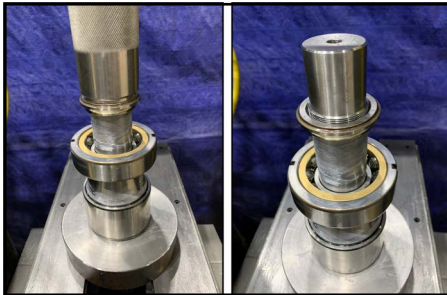
Figure 284 -Place race on shaft
