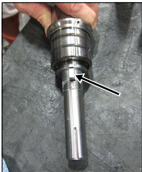
Figure 300 -Place key in key way
