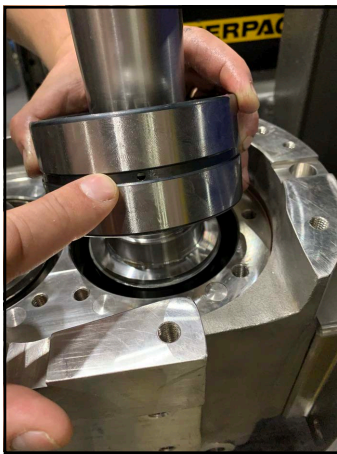
Figure 314 -Press the bearing races into the gear case
