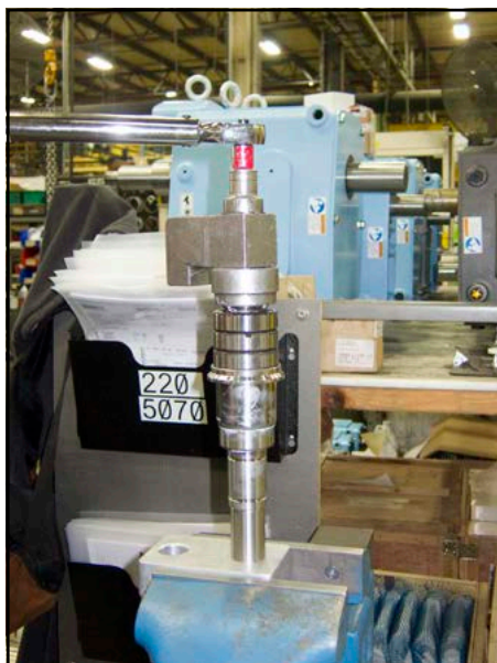
Figure 298 -Torque down locking nut
