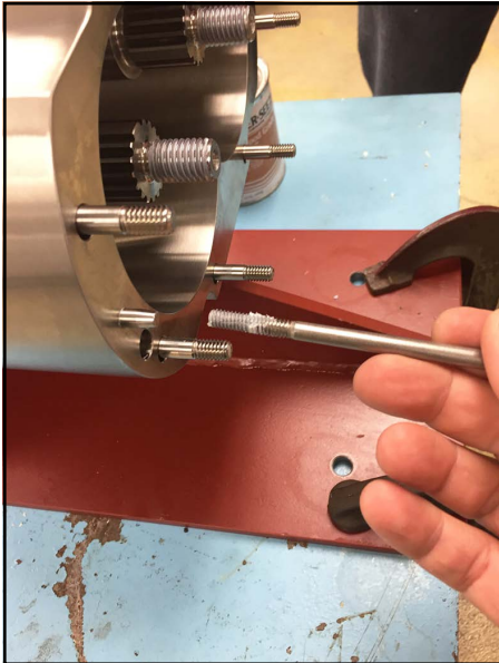
Figure 64 - Remove body retaining screws
