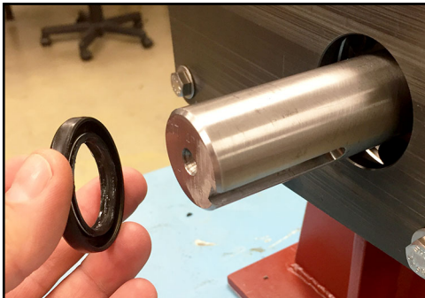
Figure 249 - Install oil seal
