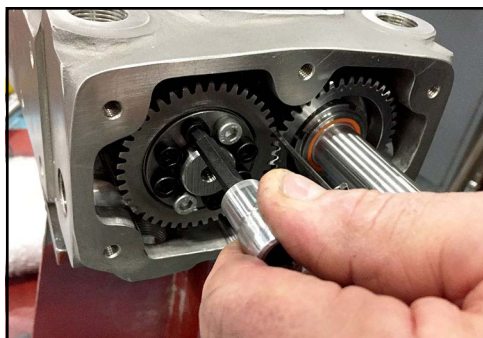
Figure 256 - Loosen bolts in locking assembly
