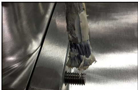
Figure 134 - Apply anti-seize to threads
