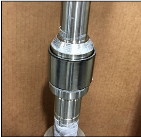
Figure 167 - Inner race installed on shaft
