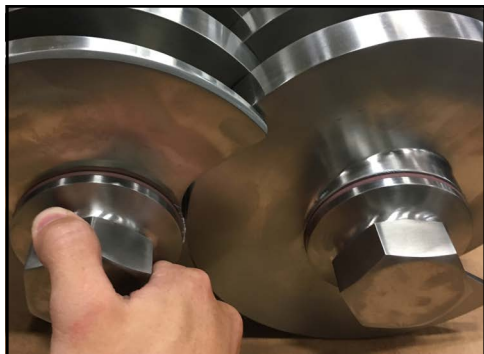
Figure 127 - Install screw nuts
