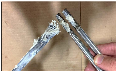
Figure 92 - Apply anti-seize to threads
