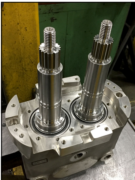
Figure 315 -Bearing outer races seated into gear case
