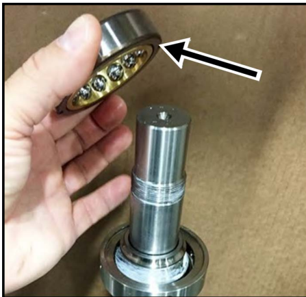
Figure 283 -Place bearing onto race
