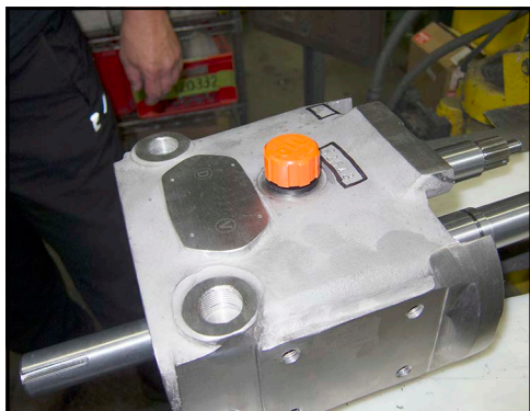
Figure 219 - Install oil breather plug
