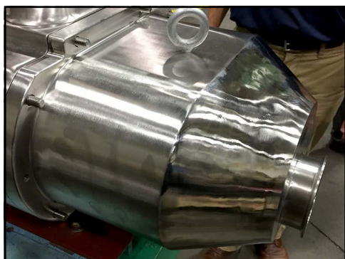
Figure 133 - Seat pump cover against pump body
