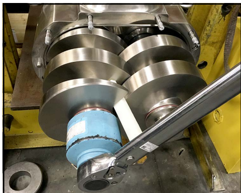
Figure 128 - Torque left screw nut
