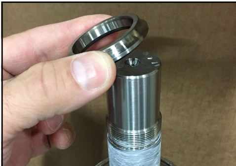
Figure 173 - Place race onto shaft
