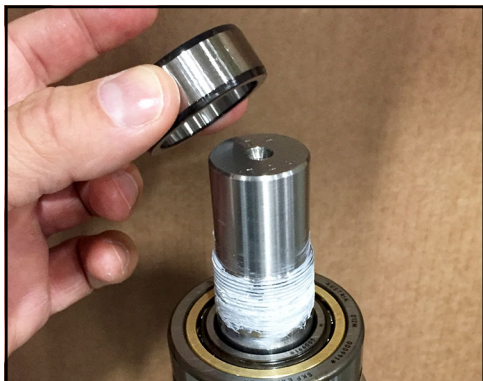
Figure 186 - Place race onto shaft
