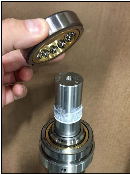
Figure 291 -Place bearing onto race
