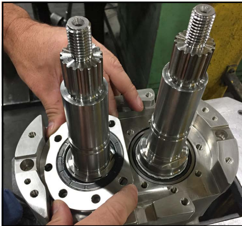
Figure 265 - Remove bearing retainer
