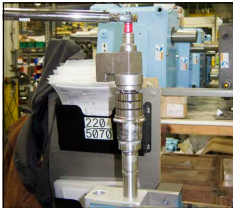
Figure 190 - Torque down locking nut
