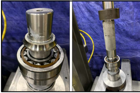
Figure 289 -Place race on shaft
