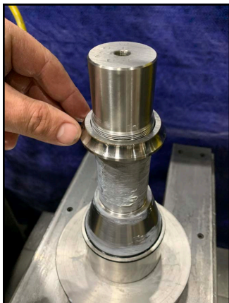
Figure 280 -Place race onto shaft
