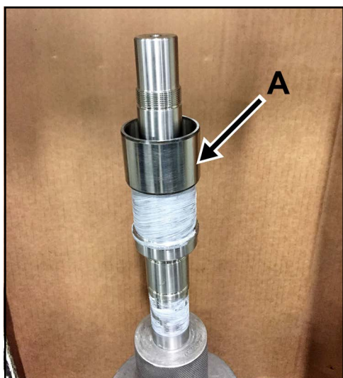
Figure 165 - Place inner race on shaft
