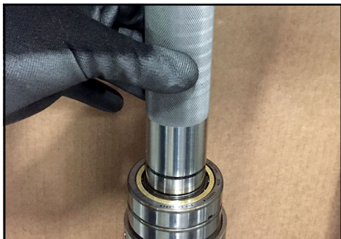
Figure 187 - Press race onto shaft
