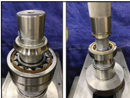
Figure 296 -Press race into bearing
