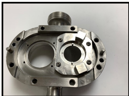
Figure 96 Seal housing installed
