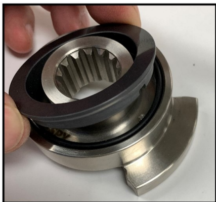
Figure 74 Remove rotary seal
