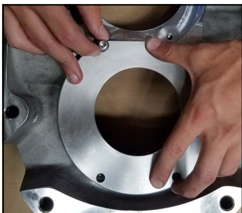
Figure 142 - Install seal housing bolts
