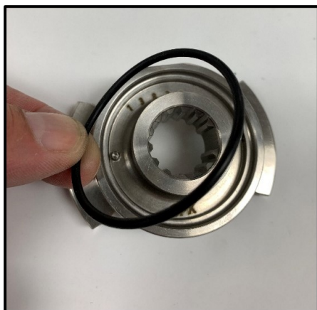
Figure 42 Remove seal O-ring
