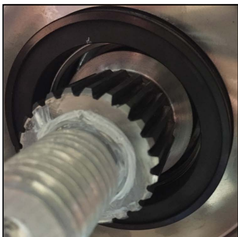
Figure 212 - Stationary seal installed
