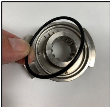
Figure 72 Install seal O-ring
