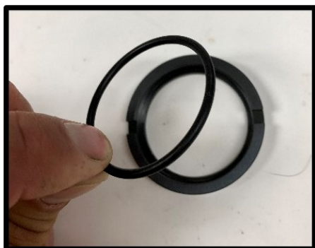
Figure 103 Install flush side rotary O-ring
