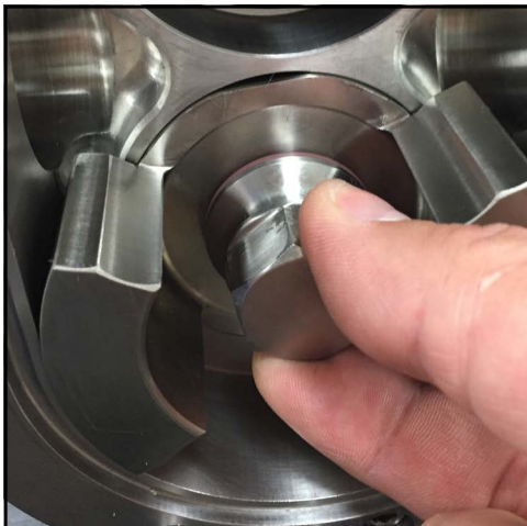
Figure 259 - Install rotor nut
