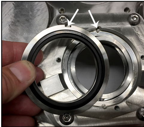
Figure 172 - Install flush-side stationary seal
