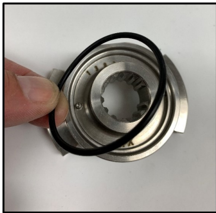
Figure 50 Install seal O-ring
