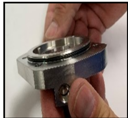
Figure 92 Install the seal housing O-ring
