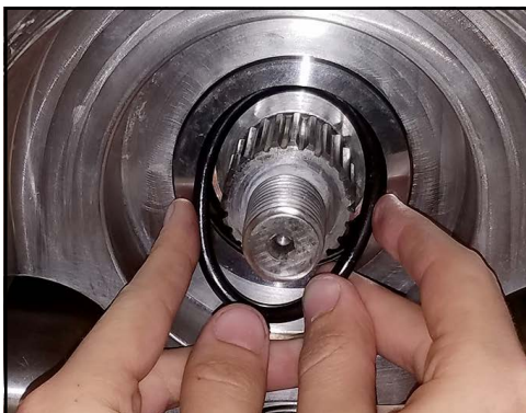
Figure 246 - Install seal O-ring
