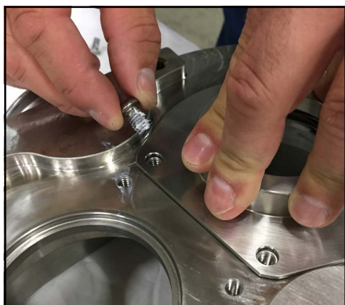
Figure 136 - Install seal housing bolts
