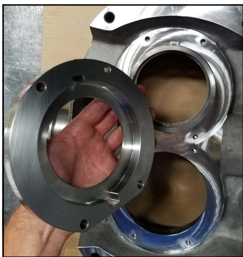
Figure 124 - Remove seal housing
