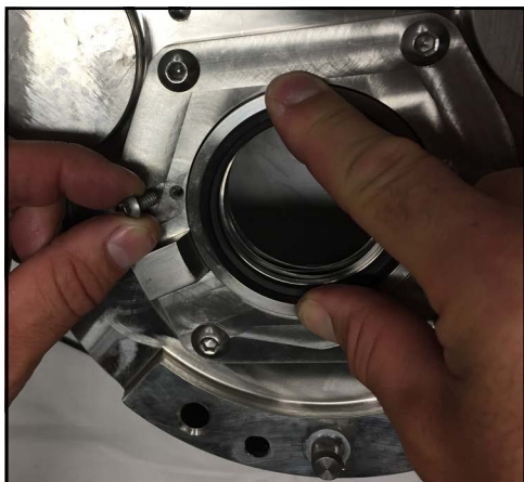
Figure 148 - Remove seal retaining bolts
