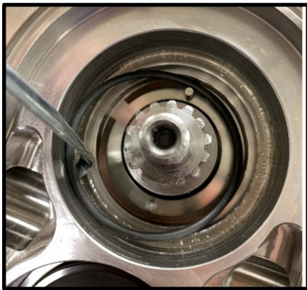
Figure 77 Remove stationary seal O-ring
