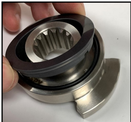
Figure 52 Remove rotary seal
