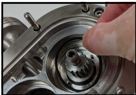
Figure 68 Install stationary O-ring
