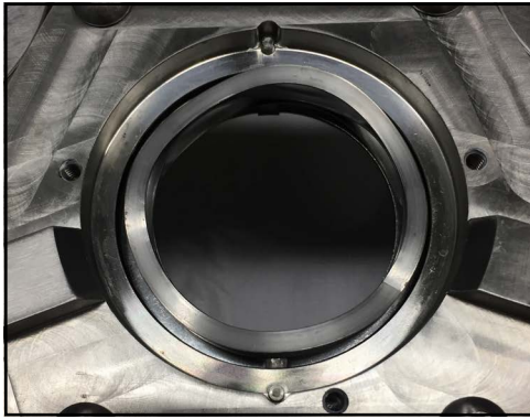
Figure 171 - Wave spring installed
