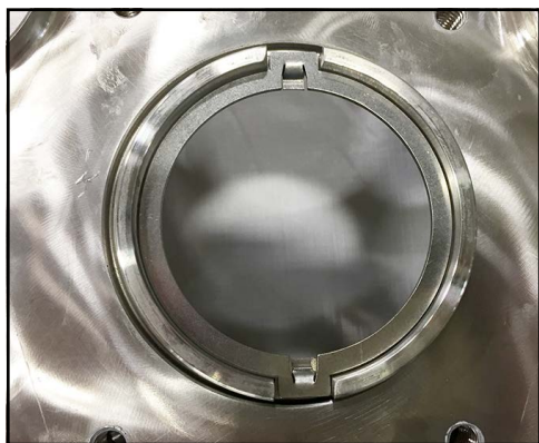
Figure 162 - Drive ring installed
