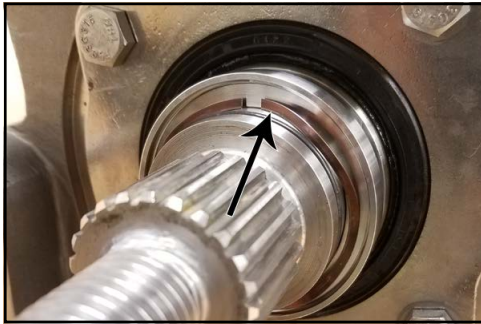
Figure 230 - Remove wave spring
