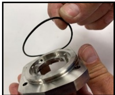
Figure 91 Double Mechanical Seal
