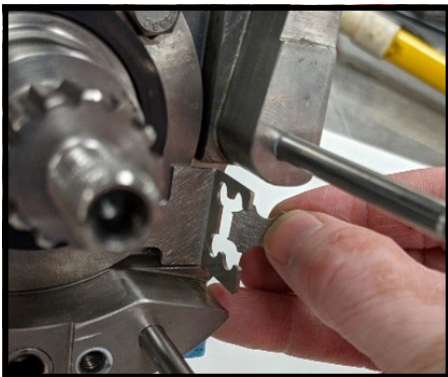
Figure 106 Break tab off finger guard
