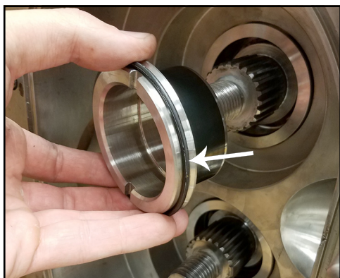
Figure 220 - Remove sleeve, O-ring
