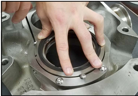
Figure 195 - Install seal retaining bolts
