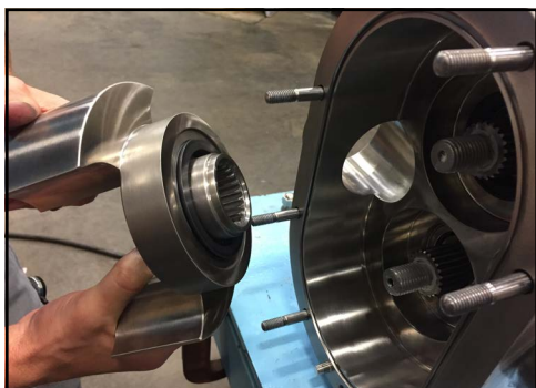
Figure 255 - Push rotor on shaft
