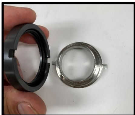
Figure 104 Install flush side rotary seal
