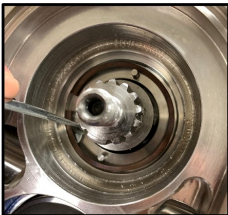
Figure 78 Remove stationary seal wave spring
