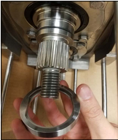
Figure 231 - Remove seal seat
