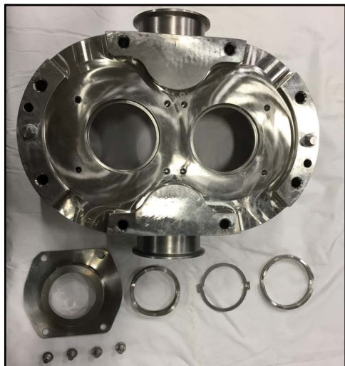
Figure 128 - Single Mechanical Seal (040-U3 shown)
