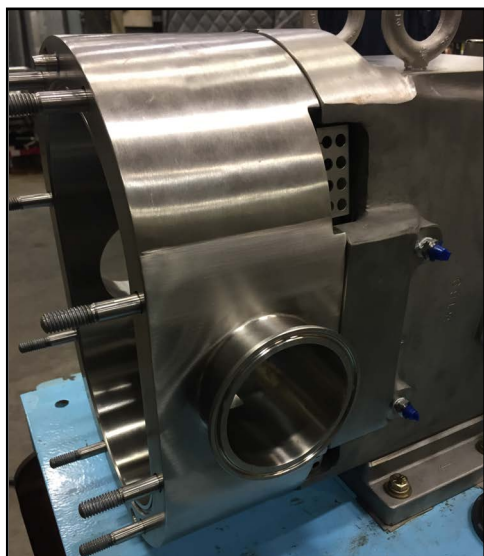
Figure 206 - Pump body installed
