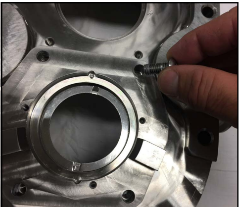
Figure 166 - Seal housing bolts
