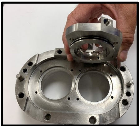
Figure 94 Install seal housing
