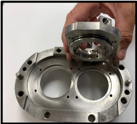
Figure 89 Remove seal housing
