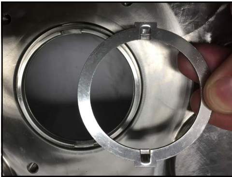
Figure 156 - Remove drive ring
