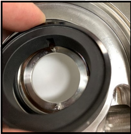
Figure 70 Install stationary seal
