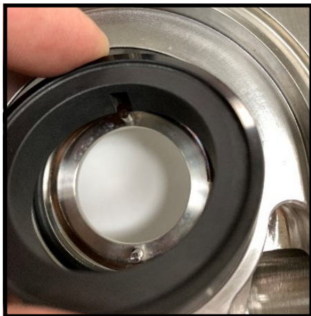
Figure 48 Install stationary seal
