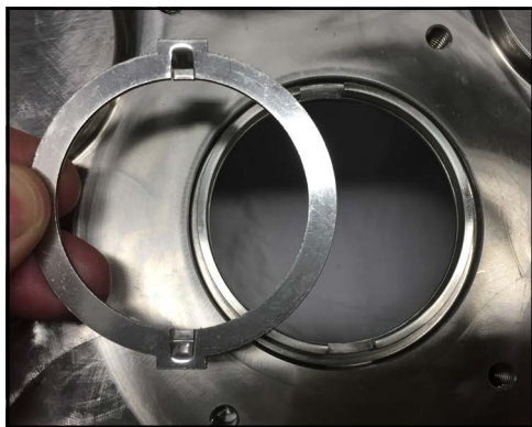
Figure 161 - Install drive ring
