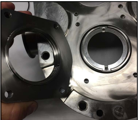
Figure 165 - Install seal housing
