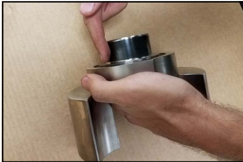
Figure 252 - Lubricate seal sleeve
