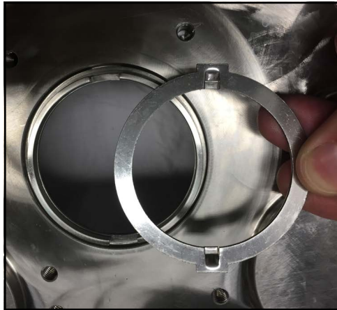
Figure 126 - Remove drive ring
