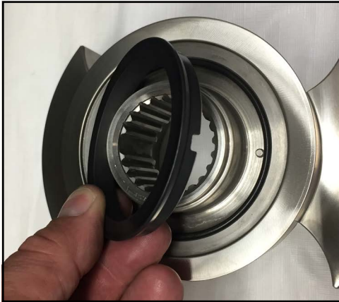
Figure 116 - Remove rotary seal
