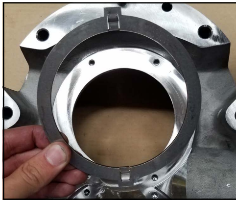
Figure 138 - Install drive ring
