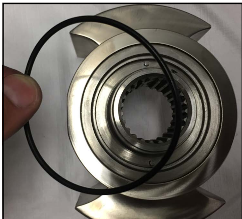
Figure 213 - Install seal O-ring
