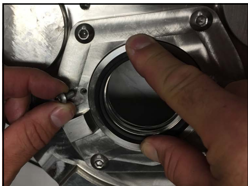
Figure 174 - Install seal retaining bolts
