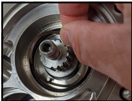
Figure 47 Install stationary wave spring
