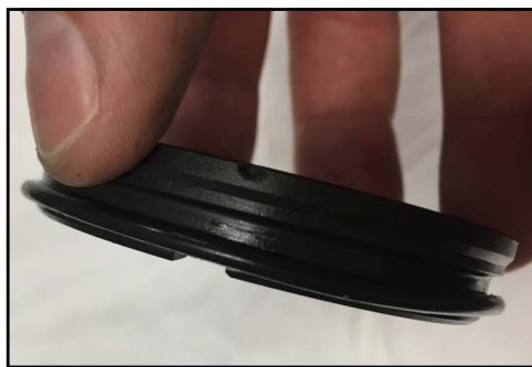
Figure 209 - Seal O-ring installed
