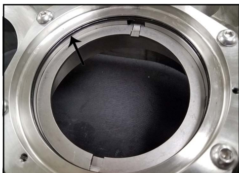
Figure 192 - Seal O-ring location
