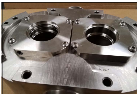
Figure 237 - Seal housings installed
