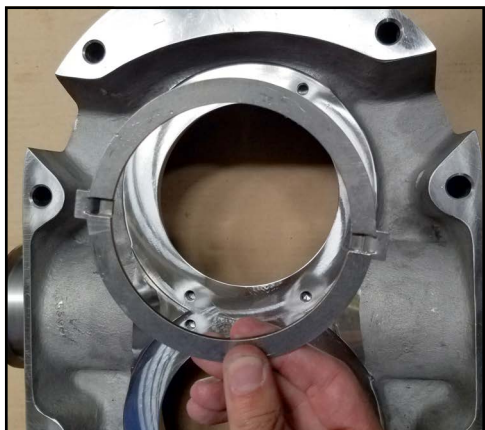
Figure 185 - Install drive ring
