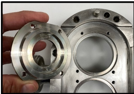
Figure 62 Install seal housing
