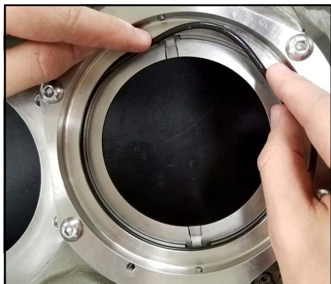
Figure 191 - Install seal O-ring
