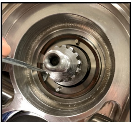
Figure 45 Remove stationary seal wave spring
