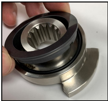
Figure 73 Install rotary seal
