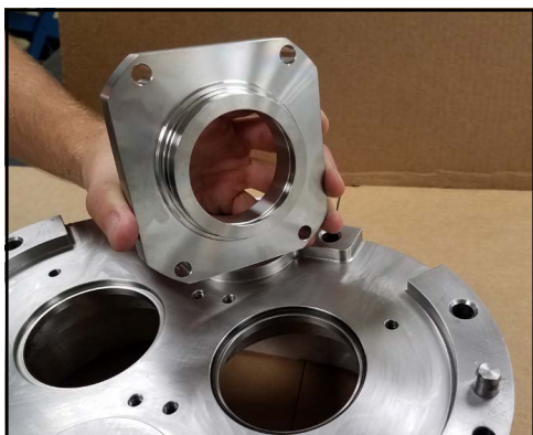
Figure 234 - Line up bolt holes
