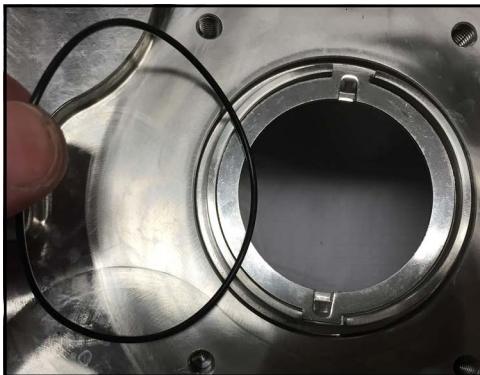
Figure 154 - Remove seal housing O-ring
