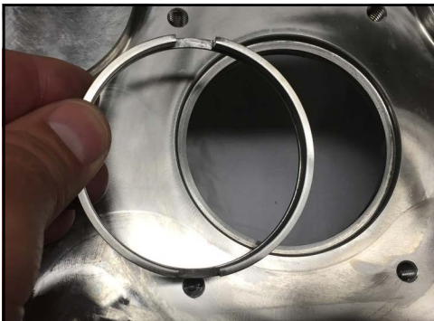
Figure 157 - Remove shaft ring
