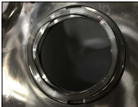
Figure 134 - Wave spring installed
