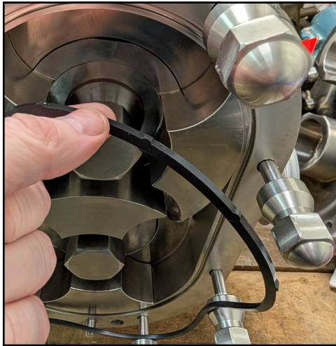
Figure 262 - Install cover gasket
