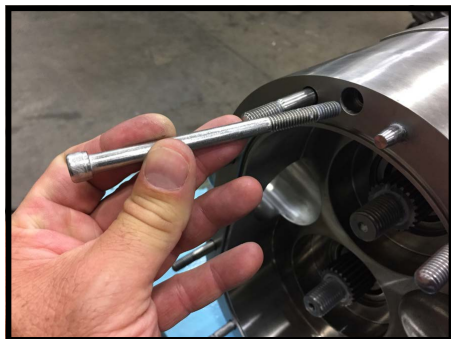
Figure 79 Remove body retaining screws
