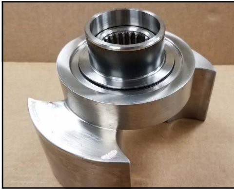
Figure 251 - Seal sleeve installed
