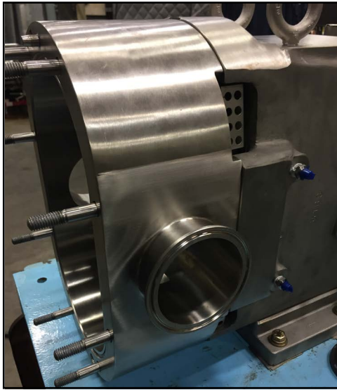
Figure 244 - Pump body installed
