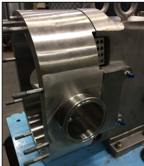
Figure 66 - Pump body installed
