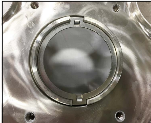
Figure 132 - drive ring installed (134-U3 and smaller
