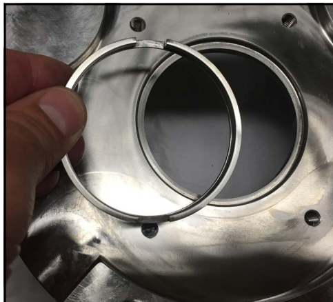
Figure 127 - Remove shaft ring
