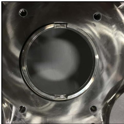
Figure 160 - Shaft ring installed
