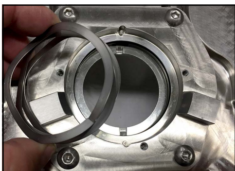
Figure 150 - Remove wave spring
