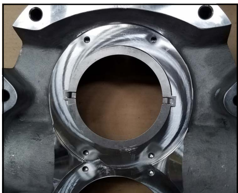
Figure 186 - Drive ring installed
