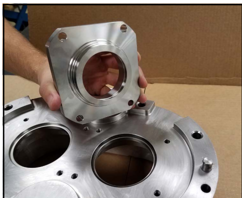
Figure 228 - Remove seal housing
