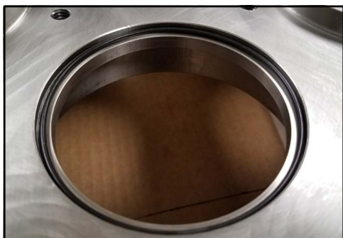
Figure 233 - Seal housing O-ring installed
