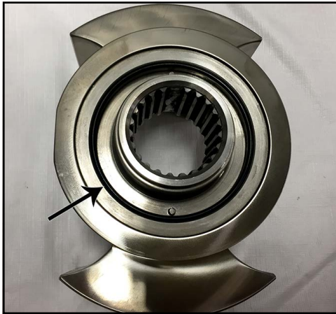
Figure 214 - Seal O-ring installed
