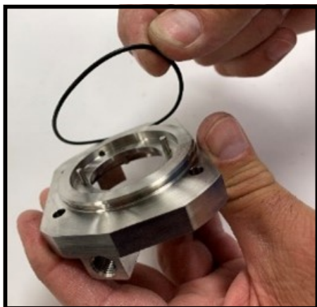
Figure 90 Remove seal housing O-ring
