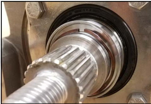
Figure 242 - Install wave spring
