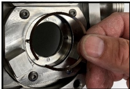
Figure 98 Install stationary seal wave spring
