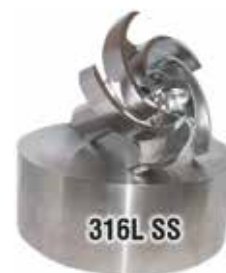
All Wet-end components are made from wrought 316SS, (UNS 31603) bar or flat stock with composition and manufacturing process controls that limit delta ferrite content to less than 5%.
