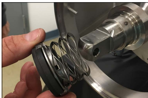
Figure 19 - Remove seal, O-ring, seal cup and spring
