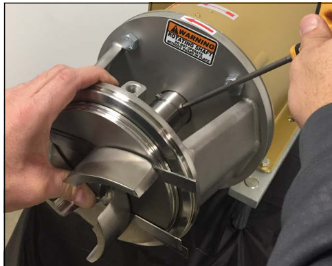
Figure 37 - Place feeler gauge, tighten setscrews
