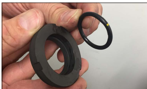
Figure 42 - Lubricate and install O-ring
