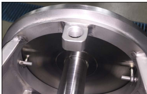
Figure 48 - Backplate pins engaged
