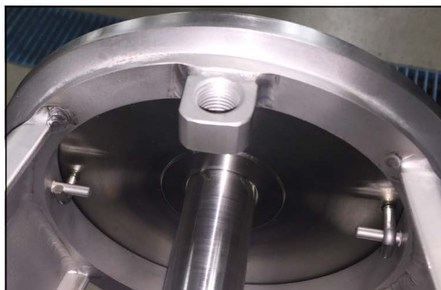
Figure 32 - Backplate pins engaged with adapter pins
