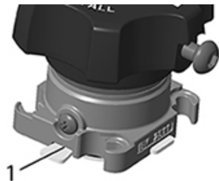
Figure 19: Body to Bonnet Mount - Potential Pinch Points
