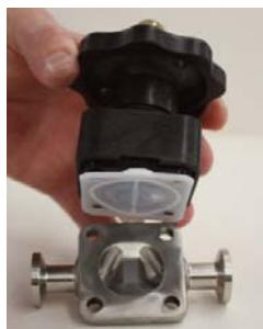
4. Unscrew the diaphragm from the compressor by turning counterclockwise..
