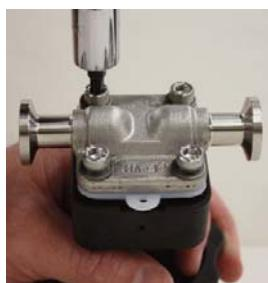
3. Lift actuator assembly from valve body.
