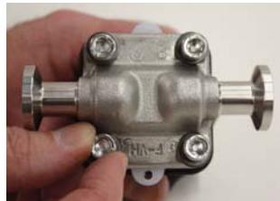
10. Tighten the bonnet fasteners in a crisscross pattern. Make multiple criss-cross passes to build up torque to the final table value. Make additional criss-cross passes using final table values to evenly tighten each fastener to within 5% of torque value.
