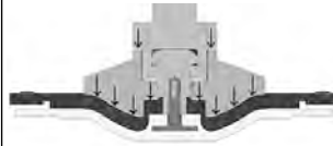
Figure 2: Compressor for Advantage 2.0 actuator
