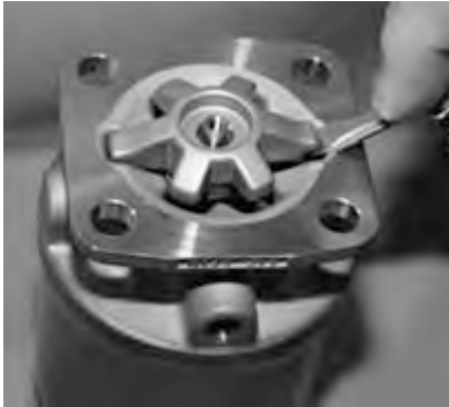
Figure 8: Remove the compressor
