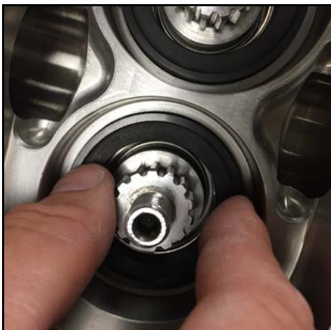
Figure 133 - Push on stationary seal
