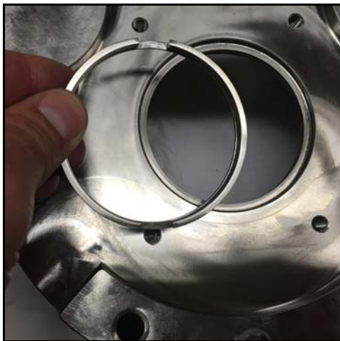
Figure 81 - Install shaft ring
