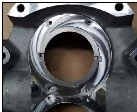
Figure 108 - Drive ring installed
