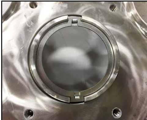
Figure 54 - drive ring installed (130-U3 and smaller)
