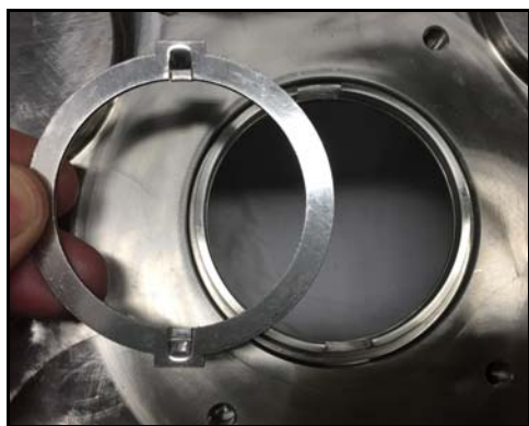
Figure 83 - Install drive ring
