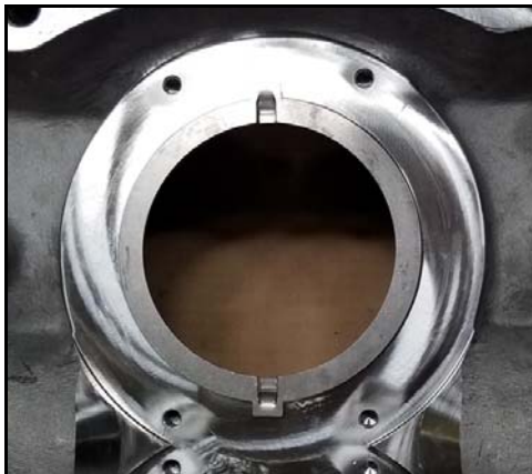
Figure 61 - Drive ring installed
