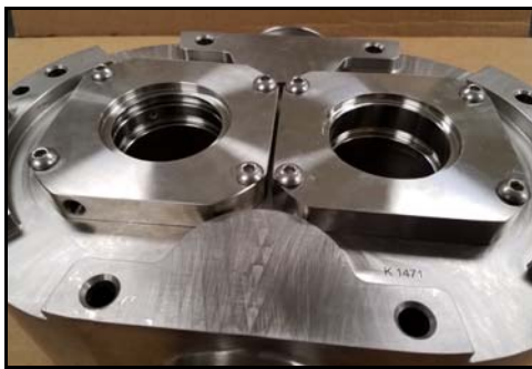
Figure 159 - Seal housings installed
