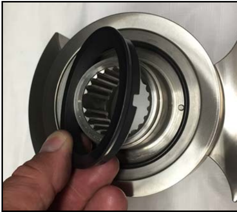
Figure 137 - Install rotary seal
