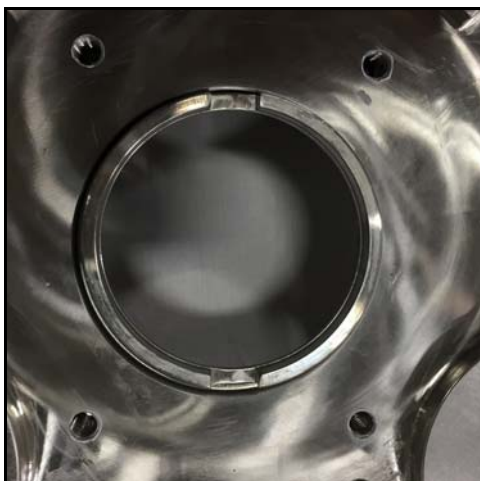
Figure 82 - Shaft ring installed
