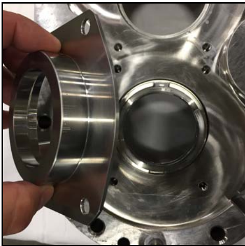
Figure 45 - Remove seal housing
