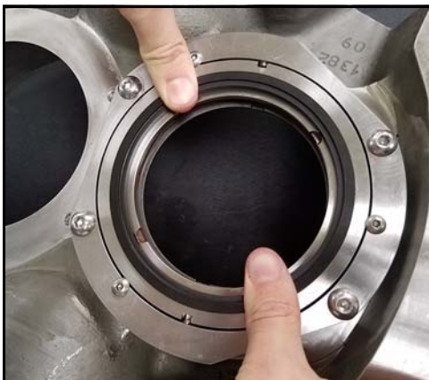
Figure 118 - Apply finger pressure
