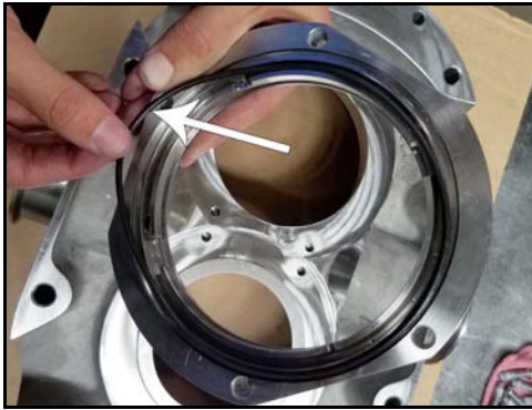
Figure 77 - Remove seal housing O-ring
