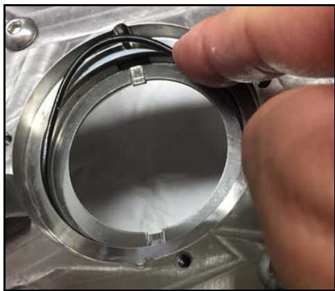
Figure 90 - Install seal O-ring
