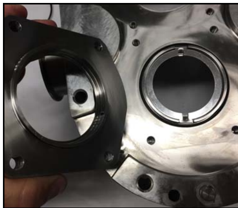
Figure 87 - Install seal housing
