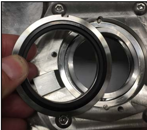
Figure 71 - Remove stationary seal
