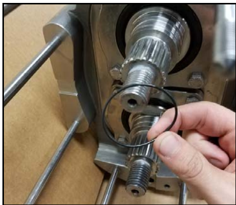
Figure 160 - Lubricate and install O-ring
