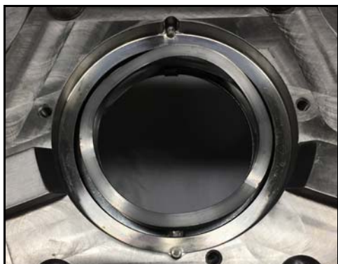
Figure 93 - Wave spring installed
