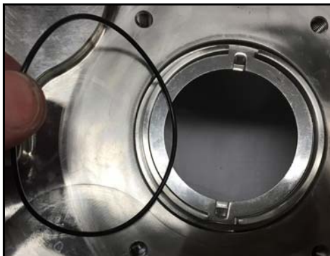
Figure 76 - Remove seal housing O-ring
