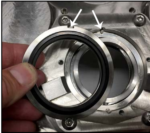
Figure 94 - Install flush-side stationary seal
