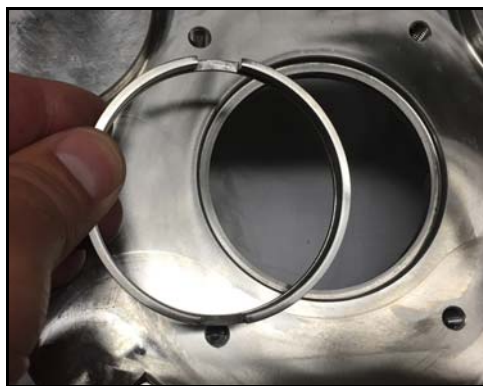
Figure 51 - Install shaft ring
