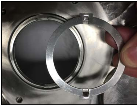
Figure 78 - Remove drive ring
