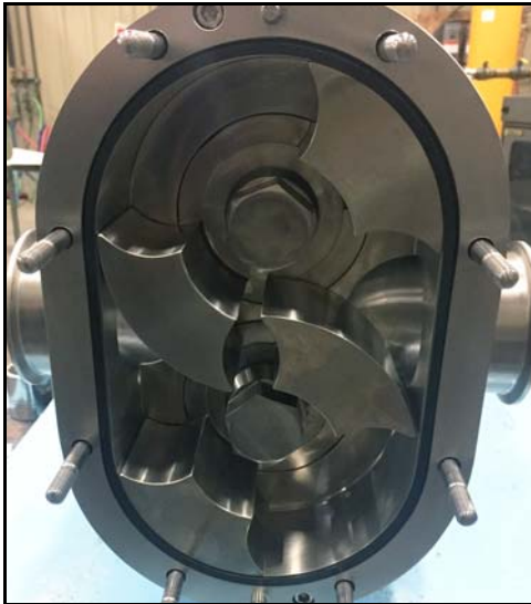
Figure 185 - Cover gasket installed
