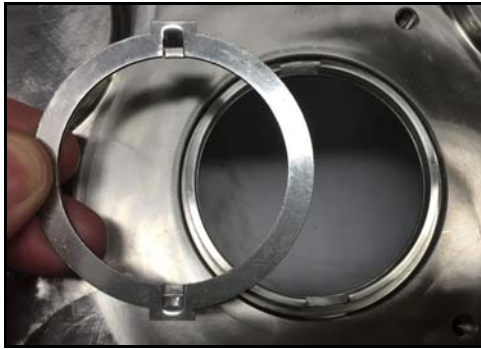
Figure 53 - Install drive ring
