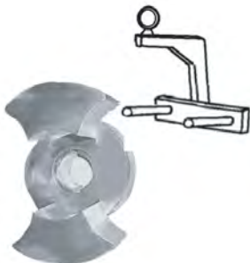
USE ROTOR REMOVAL TOOL TO REMOVE ROTORS
