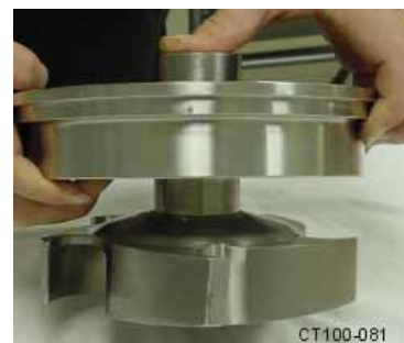
Figure 39 - Moving the Rotary Seal up the Shaft
