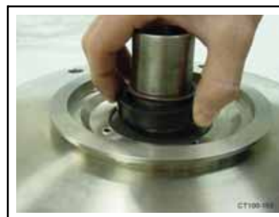
Figure 21 - Push Rotary Seal Down Releasing O-ring
