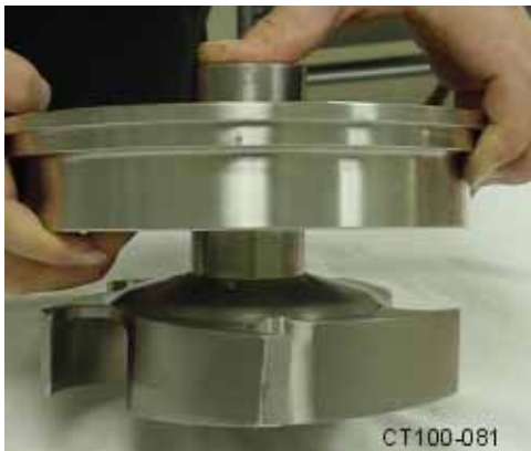
Figure 3 - Moving the Rotary Seal up the Shaft
