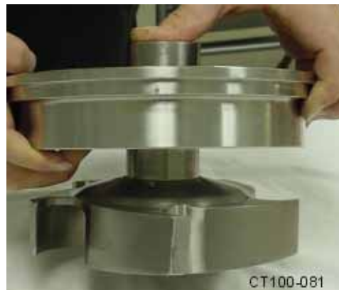
Figure 16 - Moving the Rotary Seal up the Shaft
